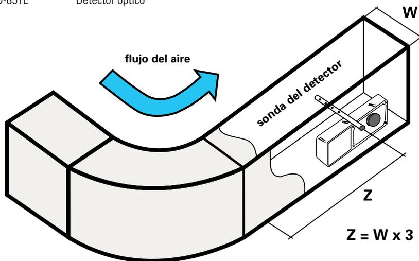
**Tubo de aspiración para conductos**
