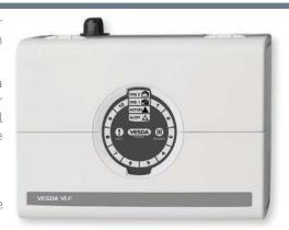
In operation, the unique Smoke Dial<sup>TM</sup> display provides the user with an instant understanding of a smoke event, even from a distance. Should a fault occur, the user simply opens the field service door and activates the Instant Fault Finder feature to determine the specific fault condition. This information can then be passed onto their fire service company, ensuring that service technicians arrive onsite fully prepared.
